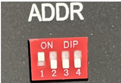
Battery DIP setting: 1: NO, 2: OFF, 3: OFF, 4: OFF
